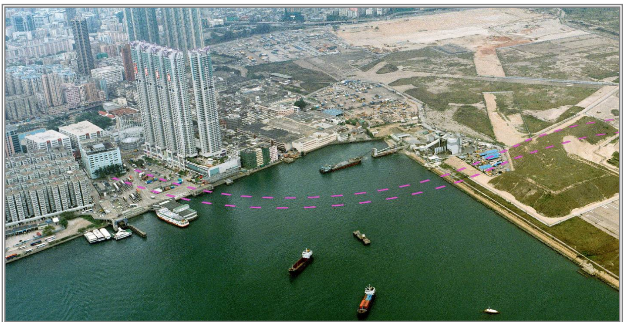
馬頭角至啓德的海底隧道 Underwater tunnel running from Ma Tau Kok to Kai Tak
